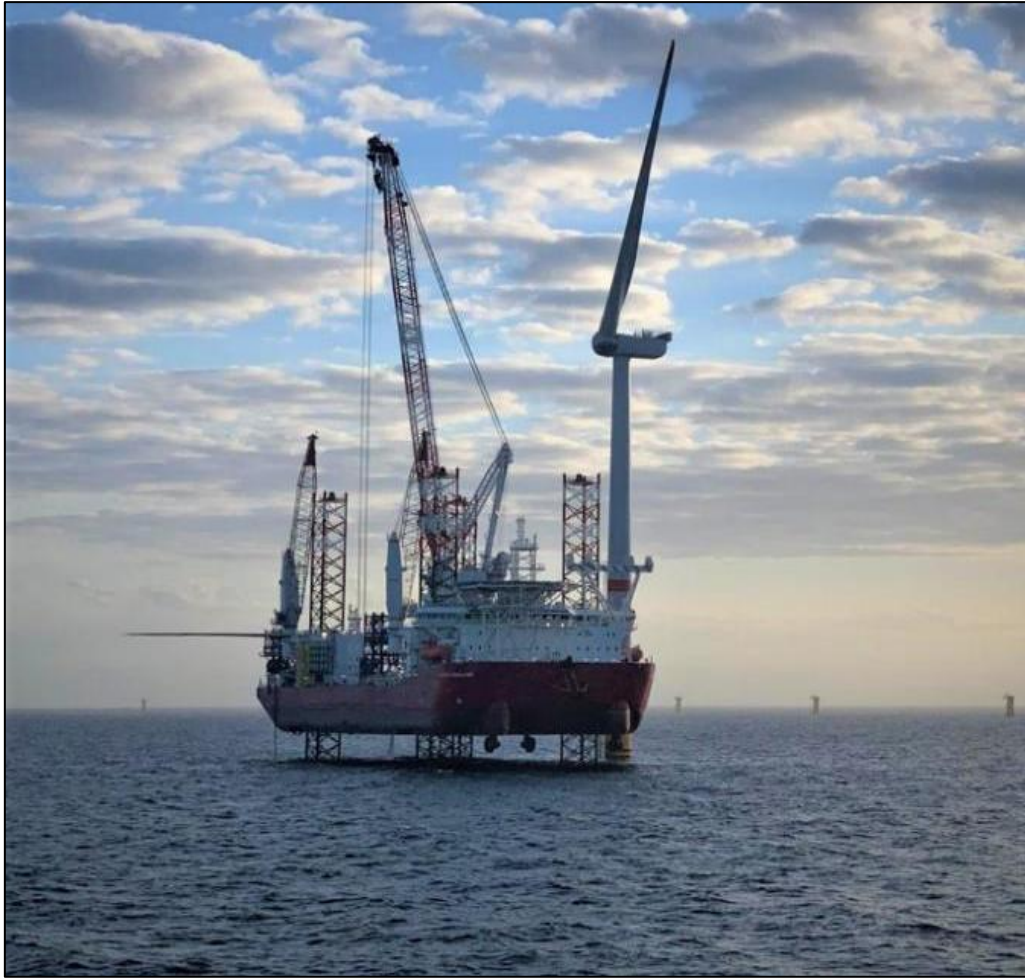
Figure 5-3: Installation vessel installing wind turbine blades.
